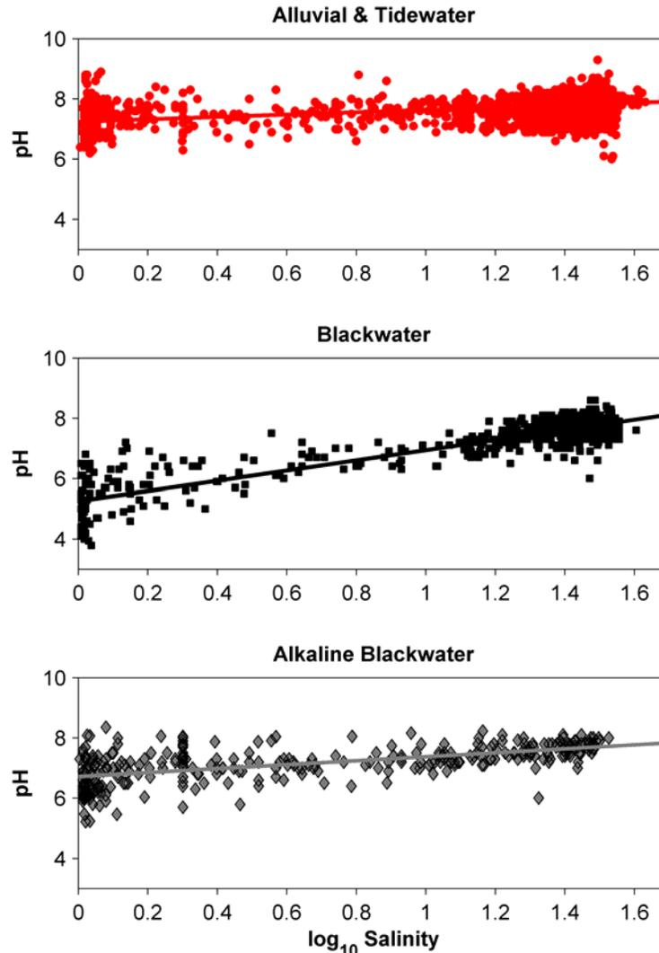
Figure 4-5. Relationships between pH and  $\log_{10}(\text{salinity}+1)$  for sites in alluvial and tidewater, blackwater, and alkaline blackwater-fed estuaries. Least-squares linear regression lines reflect “normal” pH as defined in this study.
