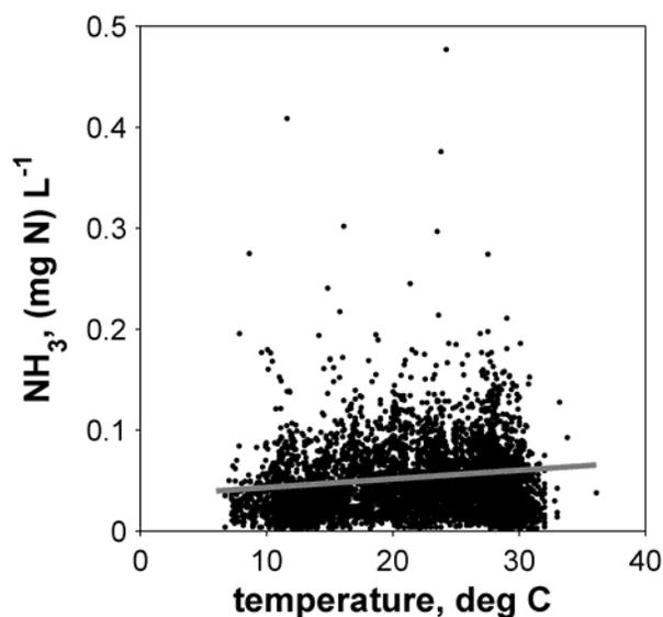
Figure 4-15. Relationship between ammonia and temperature at all stations when both parameters were sampled. Gray line represents best linear fit. 17 outliers not shown.
