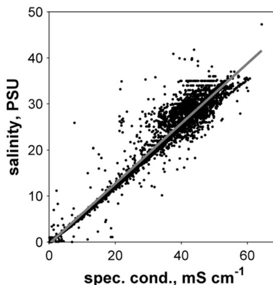
Figure 4-1. Relationship between salinity and specific conductance at all stations when both parameters were sampled. Gray line represents best linear fit.
