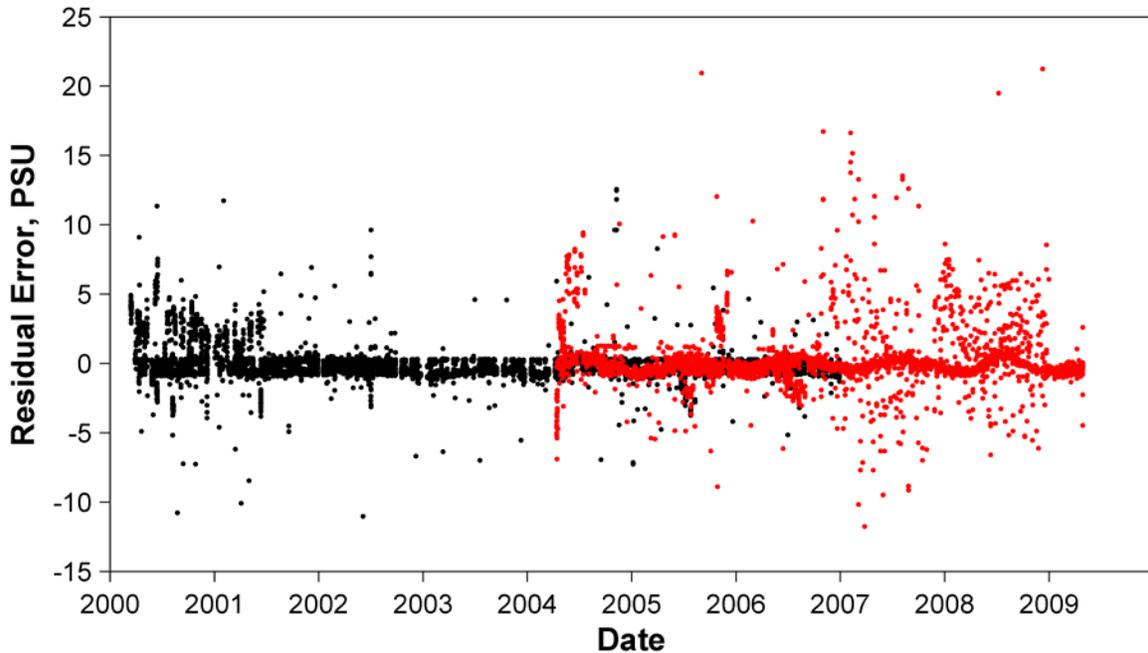
Figure 4-2. Residual error in the relationship between salinity and specific conductance. Black points are Shellfish, River, and Sound stations; red points are Beach stations.
