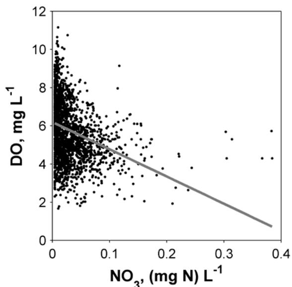
Figure 4-33. Relationship between dissolved oxygen and nitrate at Shellfish stations. Gray line represents best linear fit.
