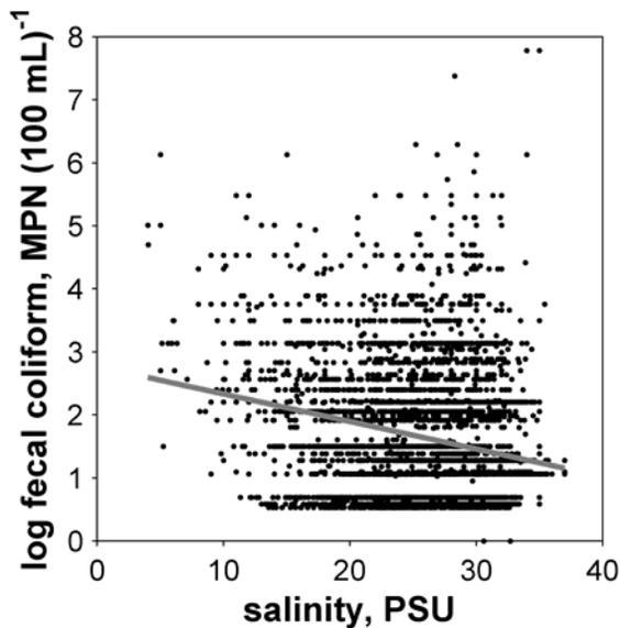
Figure 4-37. Relationship between  $\ln(\text{fecal coliform bacteria})$  and salinity at Shellfish stations. Gray line represents best linear fit.
