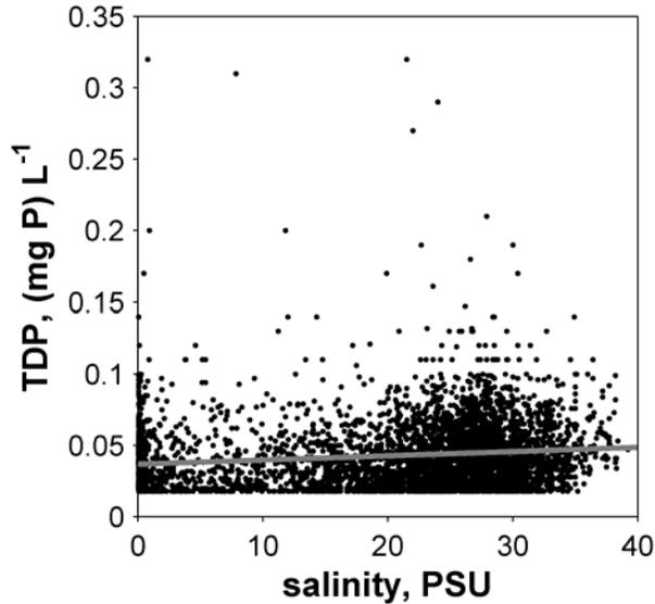
Figure 4-22. Relationship between total dissolved phosphorus and salinity at all stations when both parameters were sampled. Gray line represents best linear fit. 7 outliers not shown.
