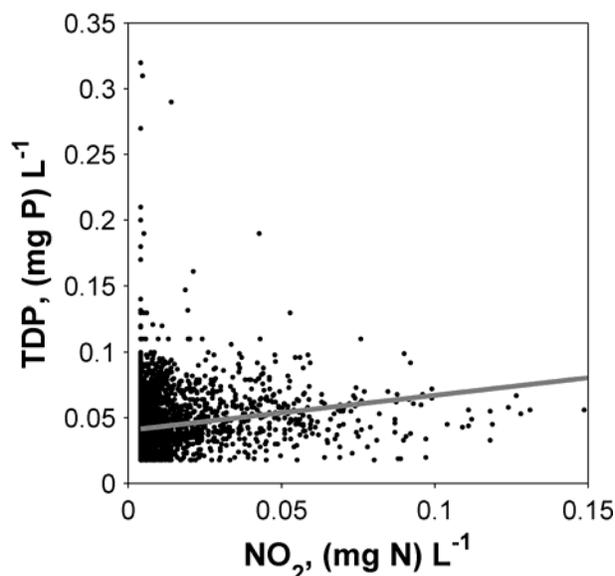
Figure 4-26. Relationship between total dissolved phosphorus and nitrite at all stations when both parameters were sampled. Gray line represents best linear fit. 6 outliers not shown.
