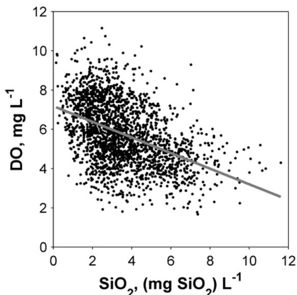
Figure 4-32. Relationship between dissolved oxygen and silicates at Shellfish stations. Gray line represents best linear fit.
