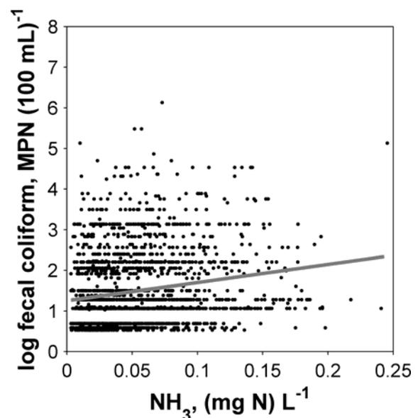
Figure 4-38. Relationship between  $\ln(\text{fecal coliform bacteria})$  and  $\text{NH}_3$  at Shellfish stations. Gray line represents best linear fit.
