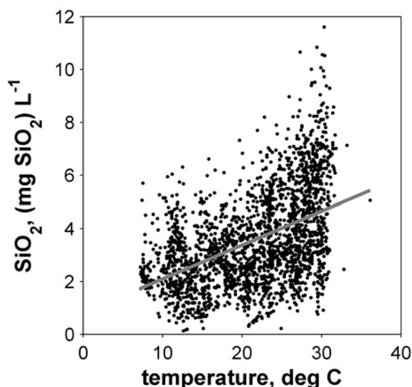
Figure 4-13. Relationship between dissolved silicates and temperature at Shellfish sites. Gray line represents best linear fit.
