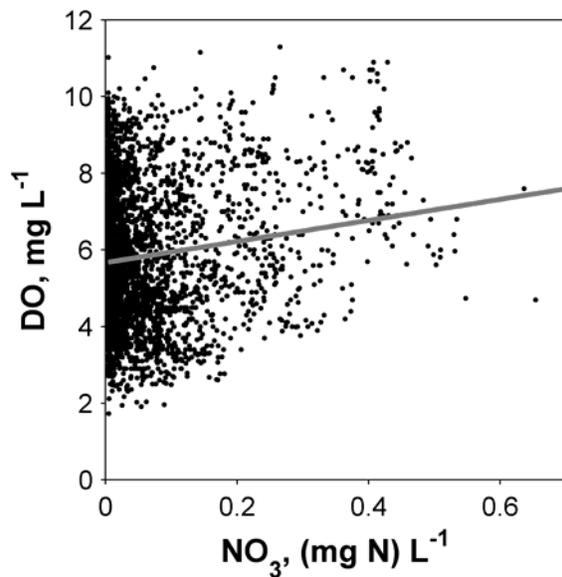
Figure 4-31. Relationship between dissolved oxygen and nitrate at River and Sound stations. Gray line represents best linear fit. 1 outlier not shown.
