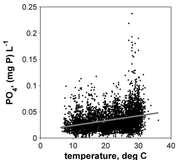
Figure 4-21. Relationship between orthophosphate and temperature at all stations when both parameters were sampled. Gray line represents best linear fit. 4 outliers not shown.
