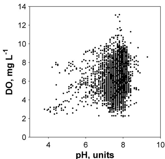
Figure 4-27. Relationship between dissolved oxygen and pH at all stations when both parameters were sampled.
