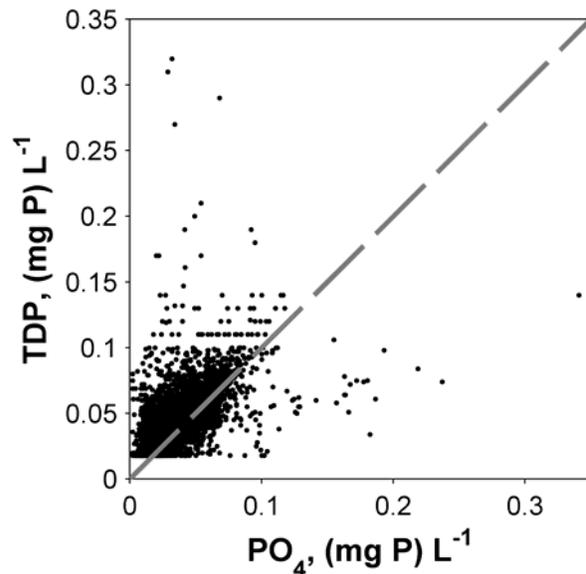
Figure 4-3. Relationship between total dissolved phosphorus and orthophosphate at all stations when both parameters were sampled. Gray dashed line represents a 1:1 relationship: all dots should be above this line. 8 outliers not shown.
