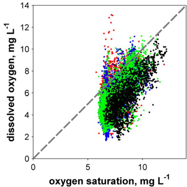
Figure 4-6. Relationship between dissolved oxygen and its saturation level based on temperature and salinity at all stations when all parameters were sampled. Colors are: red, Beach; blue, Shellfish; green, Sound; and black, River sites. Gray dashed line represents a 1:1 relationship.
