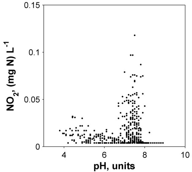
Figure 4-29. Relationship between nitrite and pH at all stations when both parameters were sampled.
