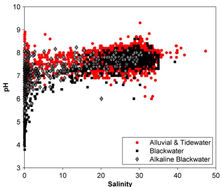
Figure 4-4. pH vs. salinity collected at all sites and times by GA DNR CRD. The relationship is different for estuaries fed by blackwater streams than it is for most other coastal locations (tidewaters and estuaries fed by alluvial streams.) Alkaline blackwater streams (i.e. the Ogeechee River) represent a special, intermediate case.
