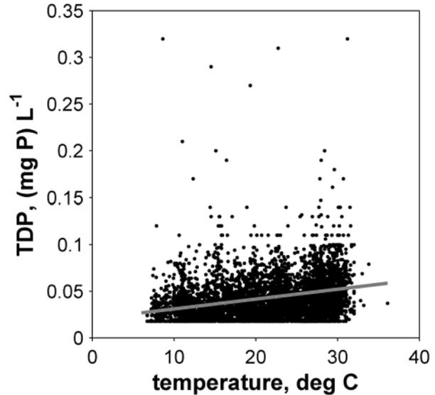
Figure 4-23. Relationship between total dissolved phosphorus and temperature at all stations when both parameters were sampled. Gray line represents best linear fit. 6 outliers not shown.
