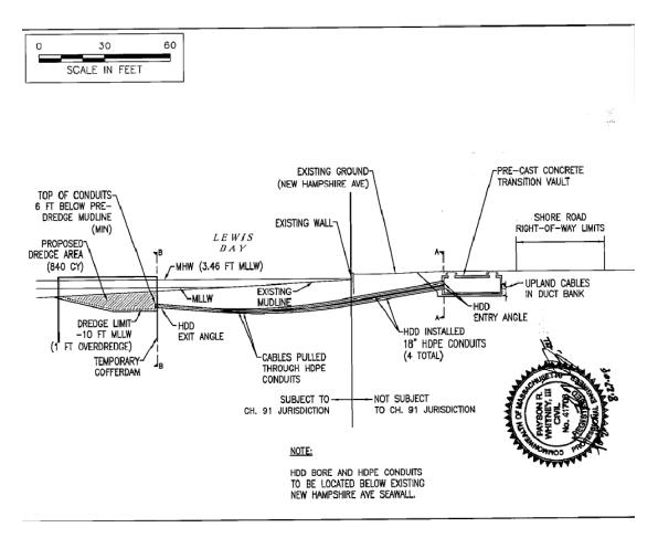
Figure 6. Profile -Proposed Landfall Conditions, Cape Wind Project (U.S. DOI BOEMRE 2008) <sup>23</sup>.
