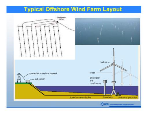
Figure 3. Generic layout of an offshore wind farm. Note that in this case the ESP is labeled as a "transformer station" (Musial  $2005^{18}$ ).
