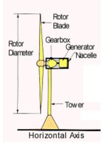
Figure 1. Basic components of a wind turbine  $(AWEA)^{15}$ .
