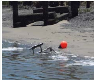
Deployed Aquadopps into Savannah River
