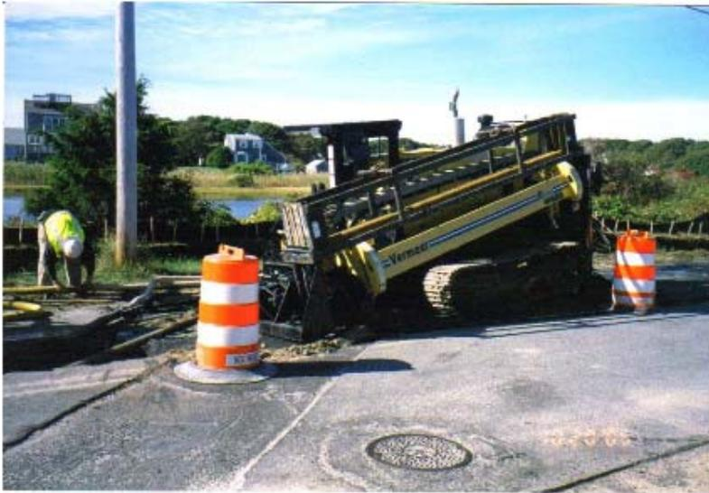
Figure 5. Example of a Horizontal Directional Drill rig for a small Nantucket Island undersea electrical transmission cable installation (not from offshore wind) (National Grid 2006).<sup>21</sup>
