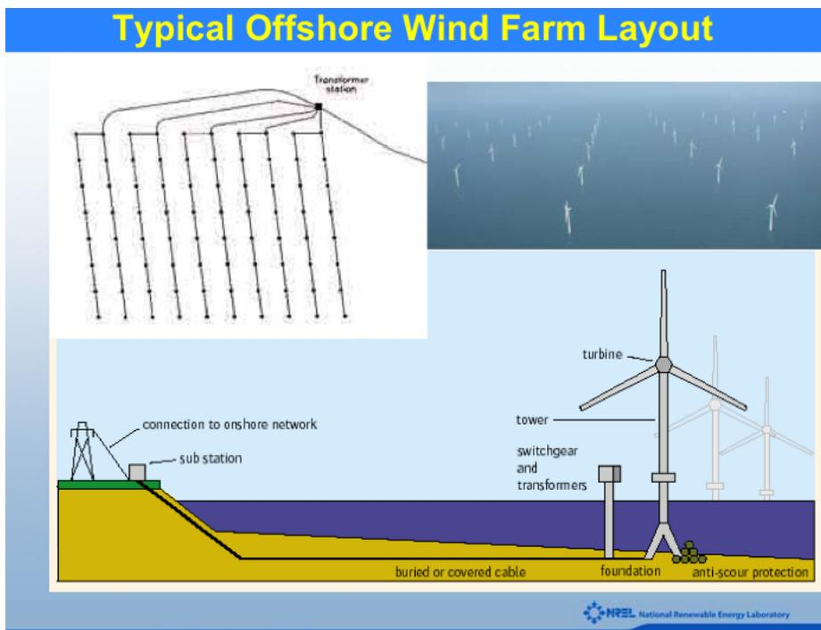
Figure 3. Generic layout of an offshore wind farm. Note that in this case the ESP is labeled as a “transformer station” (Musial 2005<sup>18</sup>).
