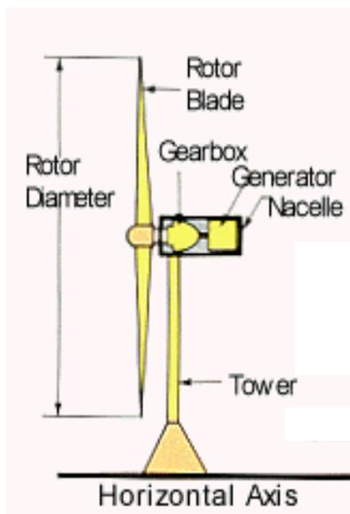
Figure 1. Basic components of a wind turbine (AWEA)<sup>15</sup>.
