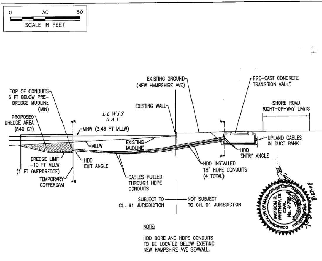
Figure 6. Profile -Proposed Landfall Conditions, Cape Wind Project (U.S. DOI BOEMRE 2008)
